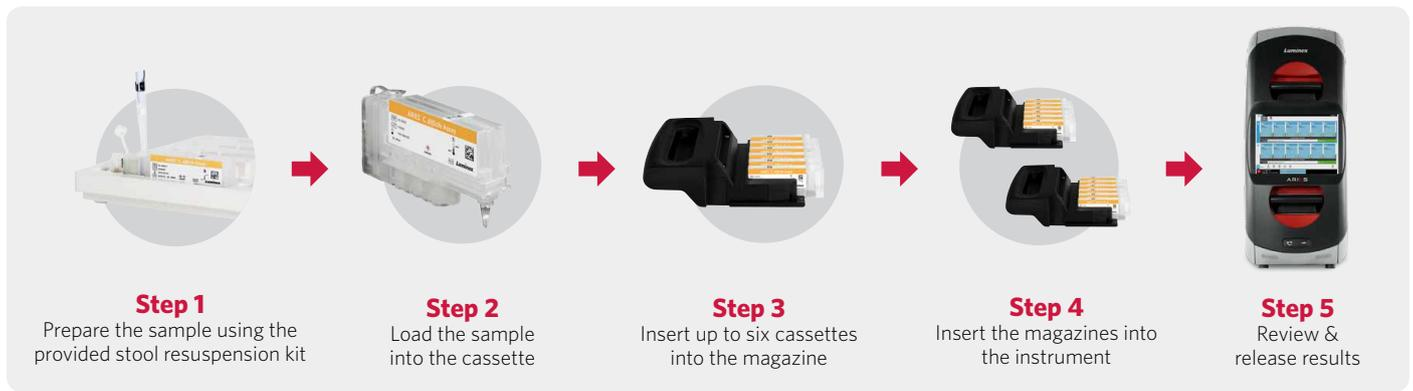
The operator prepares the sample, adds it to the cassette, puts the cassette in the magazine, loads the magazine into the ARIES® System, and the run will start automatically.
