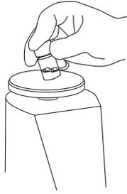
Immediately following incubation, vortex the hydrated material until pellets have completely dissolved and suspension is homogeneous.
