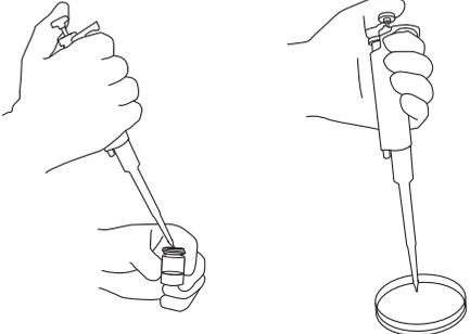
With a sterile pipette, transfer 0.1 ml of the hydrated suspension to the material being challenged (0.1 ml contains 10–100 CFU). Note: Remaining suspension can be refrigerated and used for up to 8 hours (no warming time required), with the exception of catalog numbers 0320Z and 0318Z which must be used within 30 minutes.
