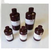
Our Secondary Reference Material (SRM) of microspheres working solution is use to control the flow cell alignment, good mechanical performance and optimal standardization of the flow cytometer.
