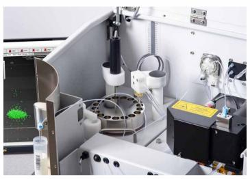
The use of an ultrasonic probe is an important feature for bacteria counting applications. The cavitation effect removes potential interfering components such as somatic cells and gives the method its high sensitivity and Signal-to-Noise ratio. The carousel is automatically cleaned before and after each analysis to eliminate carry-over. The carousel can also be easily removed from the instrument for a more thorough cleaning if necessary.
