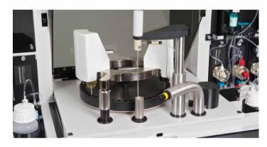
The use of ultrasonic probes is an important feature for bacteria counting applications. The cavitation effect removes potential interfering components such as somatic cells and gives the method its high sensitivity and Signal-to-Noise ratio. The carousel is automatically cleaned before and after each analysis to eliminate carry-over. The carousel can also be easily removed from the instrument for a more thorough cleaning if necessary.
